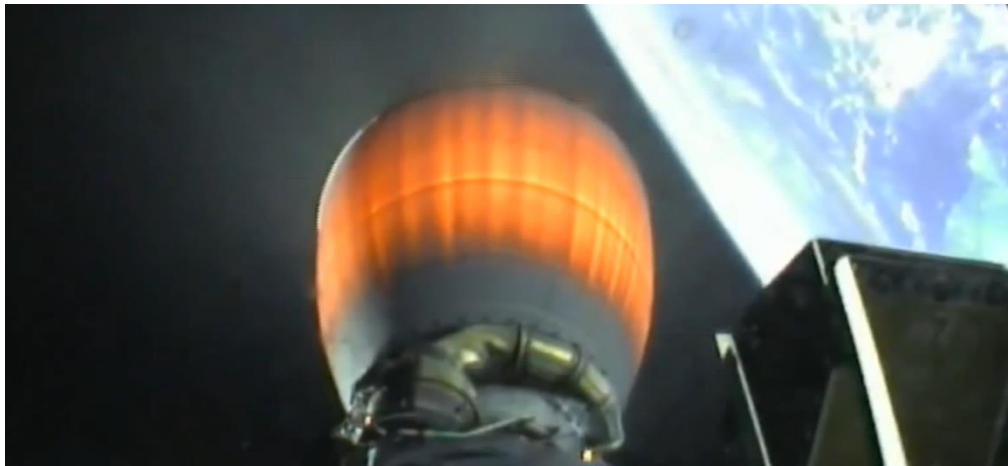
Figure 41: Merlin engine radiative cooled nozzle extension
